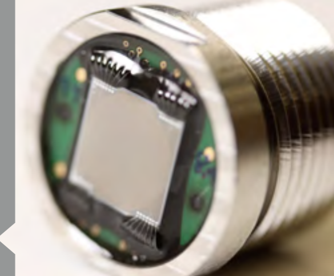
Ultrasonic sensor head based on a CMUT chip with electrically adjustable depth focus.
