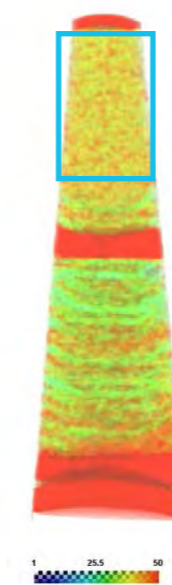
6 Distribution of the iron concentration in the layer stack (left side) and iso-concentration surfaces of iron, arsenic, cobalt, barium and oxygen showing inhomogeneities in the Ba-122 layer
