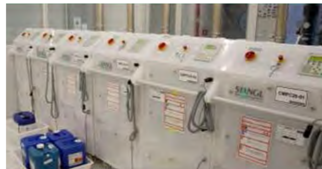
2 CMP equipment at the Fraunhofer CNT: (left) Applied Materials Reflexion LK; (right) Stangl mobile slurry systems.
