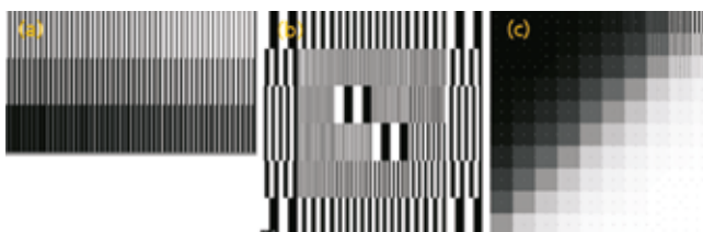
1 Structures used for process characterization. (a) Density field 1 (14 x 8 mm), (b) pitch field (14 x 14 mm), (c) density field 2 (20 x 20 mm), white: up-regions, black: down-regions. The density fields contain 18 or respectively 100 macros (2 x 2 mm) with distinct pitch and nominal densities as defined in the sketch ranging from 0 % to 100 %. The pitch field contains 36 macros (2 x 2 mm) with approximately 50 % density and a variety of pitches.
