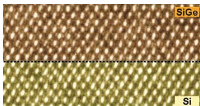
2 High resolution TEM image of the interface between epitaxial silicon germanium layer on a silicon (100) substrate.
